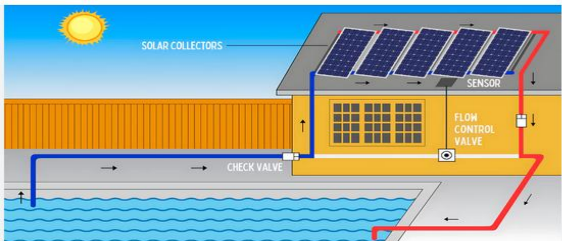
Figure 9. Swimming Pool Heating (Source: https://www.theengineeringchoice.com/what-is-solar-pool-heater/ )
